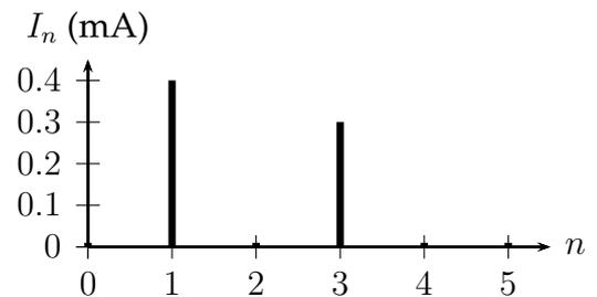
$$i(t) = C \cdot \frac{du(t)}{dt} = C \frac{d}{dt} \left[ 2 + 4 \cdot \cos \omega t + \sin 3\omega t \right] \Rightarrow i(t) = 0 - 4C\omega \sin \omega t + 3C\omega \cos \omega t$$
